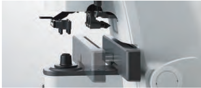
Minimize the Distance between PD Bar and Lens Support
